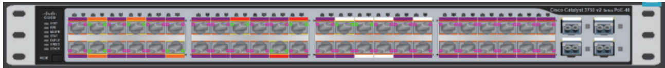
Real time graphical representation of the switch, showing recoverable parts, VLANs, port status and PoE powered switches. If skilled IT staff aren't available for remote offices, visual guidance can help an unskilled person perform patching changes.
