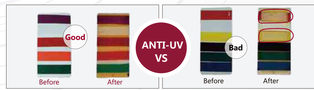
Quality color coding tape after xenon lamp exposure, after 1000 hours , product has no obvious color fading VS Inferior color coding tape after xenon lamp exposure after 1000h will has serious color fading
